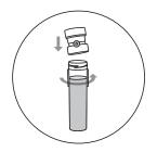
Screw the *Digi*FILTER (using the end with the plug) onto a 50 ml *Digi*TUBE containing a cooled sample.
