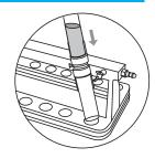
Flip the tube-filter assembly over so that the tube containing the sample is now on top. Attach the assembly to the manifold, inserting the valve into the filter port.
