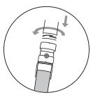
Screw a clean DigiTUBE onto the opposite end of the DigiFILTER.
