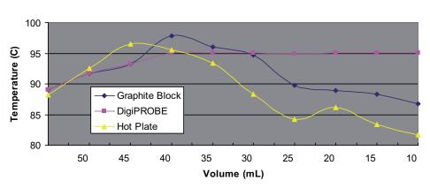
This graph depicts the sample temperature in °C, as the volume in ml decreases during the sample digestion process. Shown here is the temperature stability obtained when using the DigiPROBE as opposed to traditional heating methods such as the hot plate or the graphite block alone. As the sample volume decreases, the sample temperature is constant at 95 °C, thus showing that the temperature reading is independent of the volume in the sample tube when using the DigiPROBE during digestion.
