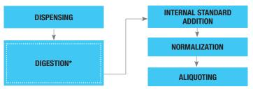
\*Digestion - Not performed by the Sample Handler. Use *DigiPREP* block digestion system (page 20) or *NovaWAVE* microwave digestion system (page 50)
